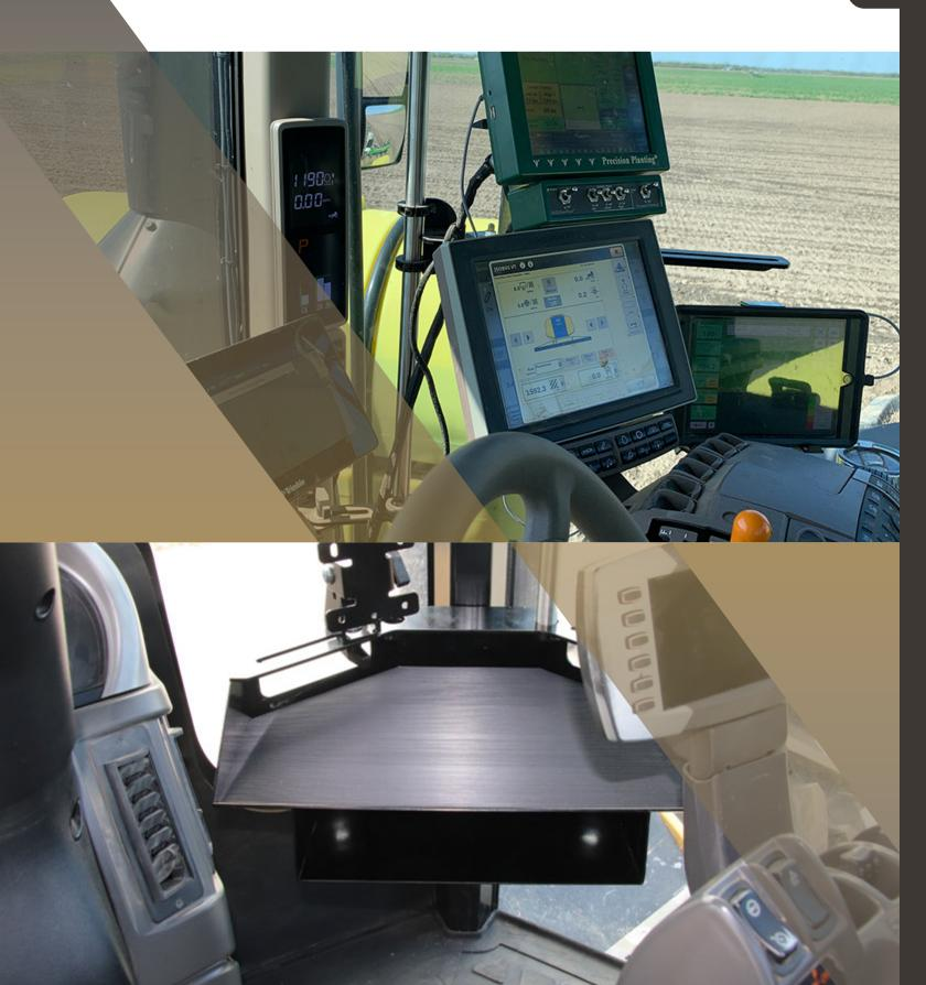
Lankota's Monitor Bracket systems are built to securely hold your monitors where you want them. They are designed to allow incredible customization. With cord storage in mind, this bracket system offers a variety of attachments to suit your exact cab needs. Lankota offers multiple bracket options for a variety of tractors and sprayers.
