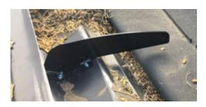
Helps the crop feed evenly to the feeder house and avoid loss or plugging under the belts.
