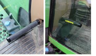
Lankota's Combine Footrest will help diminish the leg fatigue and cramping associated with long hours sitting in machinery. Fitting John Deere® combines, this kit installs in minutes using the existing bolts for the steering column.
