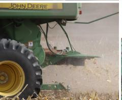
The Lankota Tailboard Spinner is a completely assembled tailboard spinner with bottom blades and top tailboard cups. The kit contains all the galvanized steel cover plates and poly, fully assembled and ready to go. The Lankota Tailboard Covers will extend the life of the factory poly tailboard spinner and provide improved durability.
