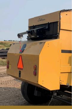
Use the Lankota Net Wrap Assist system to eliminate the backbreaking job of loading net wrap into your baler. Using 12 volt DC power from the tractor, winch net wrap into place with the push of a button. Easily and safely getting you back in the seat for more baling.
