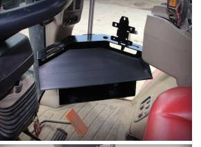
Lankota Corner Cubbies add up to 4 square feet of usable storage area. They come with a washable vinyl mat; preventing papers, folders, or cell phones from sliding around while operating the machine. Lankota offers Corner Cubby options for Case IH®, New Holland® and Challenger® tractors.
