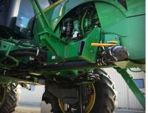
The Lankota Front Fill Kit allows you to fill your John Deere sprayer without the need to fold in the booms, allowing for more spray time with less fill time. Kits are equipped with a pump selector switch along with 3" plumbing, allowing all fill operations to be completed from the front of the sprayer.
