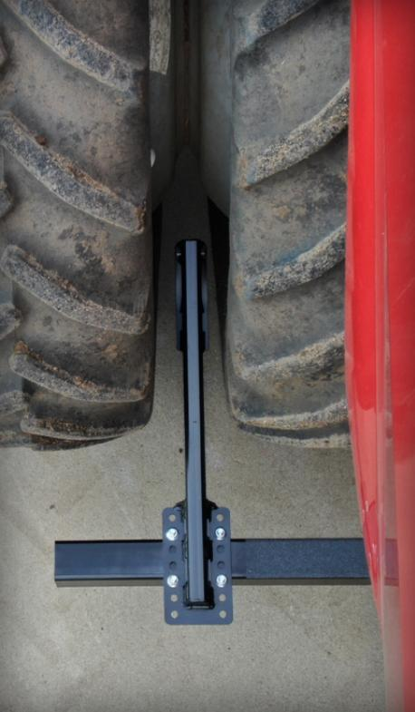
Lankota's Combine Mud Scraper System will keep your combine's front duals clean in muddy field conditions. The rugged, simple design allows for quick & easy "bolt on" installation, along with acres of continuing durability. Fully adjustable to fit any tire size and configuration, the mud scraper fits most Case IH® & New Holland® combines.
