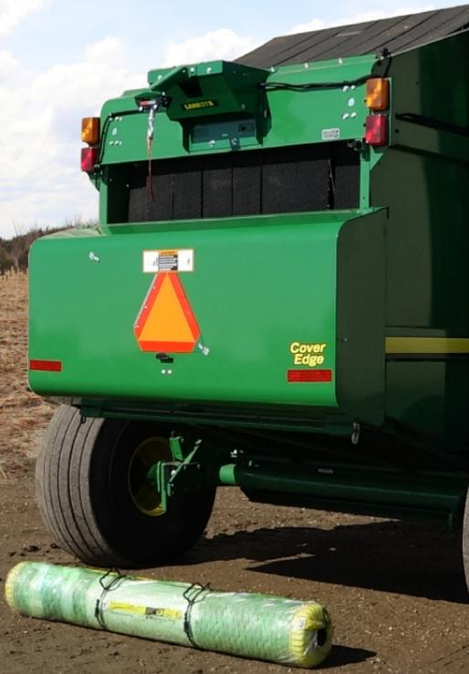
Use the Lankota Net Wrap Assist system to eliminate the back-breaking job of loading net wrap into your John Deere® baler. Using 12 volt DC power from the tractor, winch net wrap into place with the push of a button. Easily and safely getting you back in the seat for more baling.
