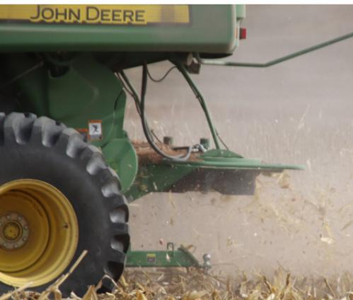
The Lankota Tailboard Spinner is a completely assembled tailboard spinner with bottom blades and top tailboard cups. The kit contains all the galvanized steel cover plates and poly, fully assembled and ready to go. The Lankota Tailboard Covers will extend the life of the factory poly tailboard spinner and provide improved durability.
