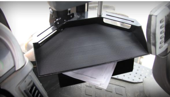
Lankota Corner Cubbies add up to 4 square feet of usable storage area. They come with a washable vinyl mat; preventing papers, folders, or cell phones from sliding around while operating the machine. Lankota offers Corner Cubby options for Case IH®, New Holland® and Challenger® tractors.
