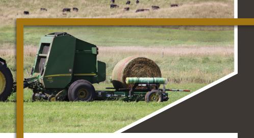
The fully automated Bale Buggy carries one bale while the second bale is being made. The Bale Buggy fits late-model John Deere, Case IH, and New Holland 5 Foot large round balers.
