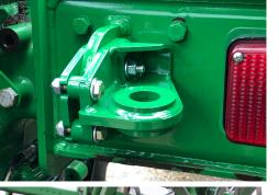
Lankota's Sprayer Tow Brackets give you peace of mind when towing your John Deere selfpropelled sprayer. The shear bolt protected system is engineered to reduce the possibility of damage to the frame. Load matched clevises and tow sling distribute the weight evenly across tow points. Brackets are included to allow towing capabilities from the front and back.
